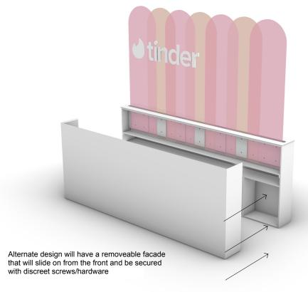
An alternative to dropping the skin/sheathing over the top of the fins is to fabricate a "U" shaped piece that can slide on from the front. The caveat with this is it will leave a small seam on the top edge where the horizontal surface meets the vertical sides.
